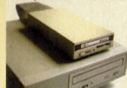
The CDPlus and SyQuest EZ135 drives. The IDE Zip Drive is the same size as the EZ135
